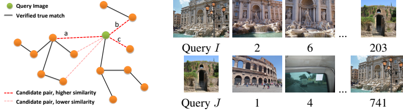
(a) Illustration of entropy-descent strategy of choosing edges to verify. The algorithm will pick edge a to verify, as it is strong and spans large CCs.
